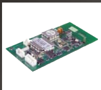
SDR-500M: Additional UHF 16ch Mic Receiver (Factory fitted only)
