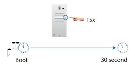
Switching between static and dynamic IP address
