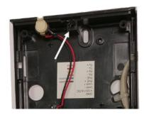
At the marked point insert the crimped cable.
