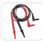
Set consisting of 1 red and 1 black extra flexible, double insulated silicone lead, 0.75 mm<sup>2</sup>, 100cm. Equipped with 4mm banana plugs with protective cover and test probe with the option of mounting alligator clips, etc.
