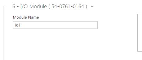
• Module name - set the module name for input/output specification in the SetOutput, GetInput and InputChanged objects in Automation.
