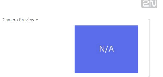
The Camera Preview window displays the current image received from an external camera. If the external camera is disconnected or configured incorrectly, the N/A characters are displayed on a blue background.
