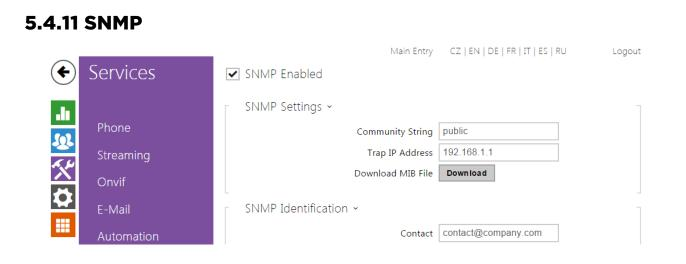
The **2N Helios IP** intercoms integrate a remote intercom supervision functionality via the SNMP. The integrated SNMP agent becomes available when the **Enhanced Integration** licence key is added. The intercoms support the SNMP version 2c.
