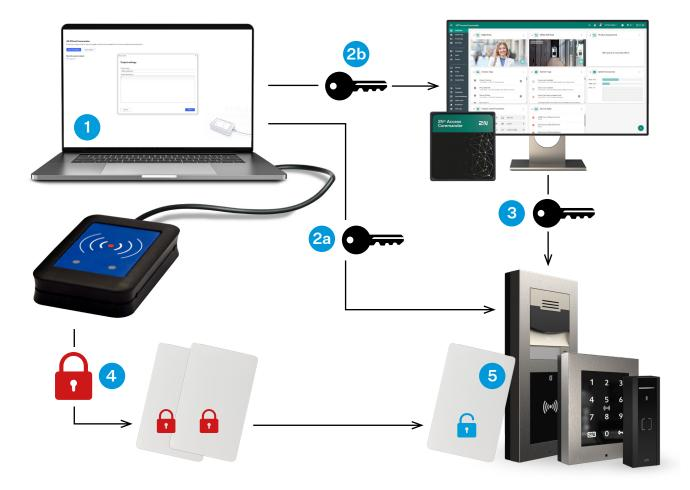
The heart of the entire solution is **2N**<sup>®</sup> **PICard Commander** – a software application that allows administrators to create a unique cryptographic keyset for every site **1**. Keysets are based on the **main encryption key (MEK):** from which encryption keys for encoding credentials and reading keys are derived.
