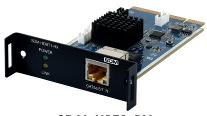
SDM-HBT1-RX HDBaseT1 Receiver SDM Module
