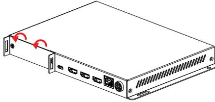
(2) Completely unscrew both screws.
