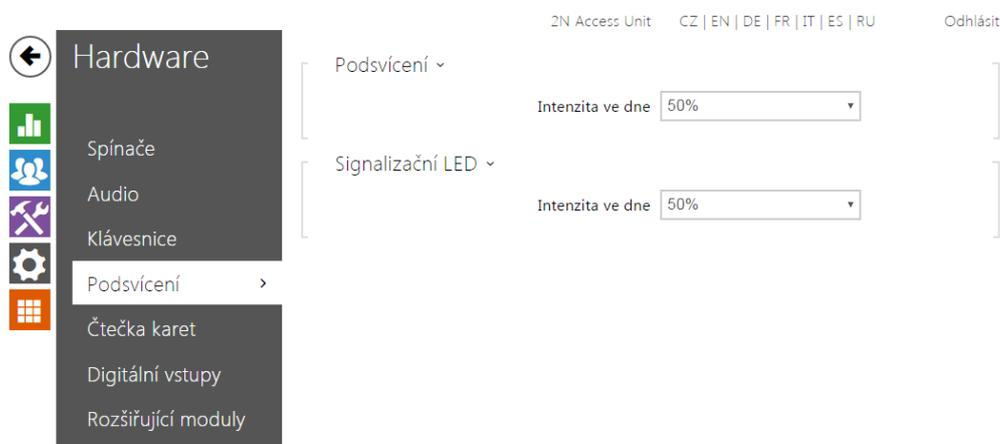
This tab helps you control the backlight level of buttons and brightness of signalling LEDs.
