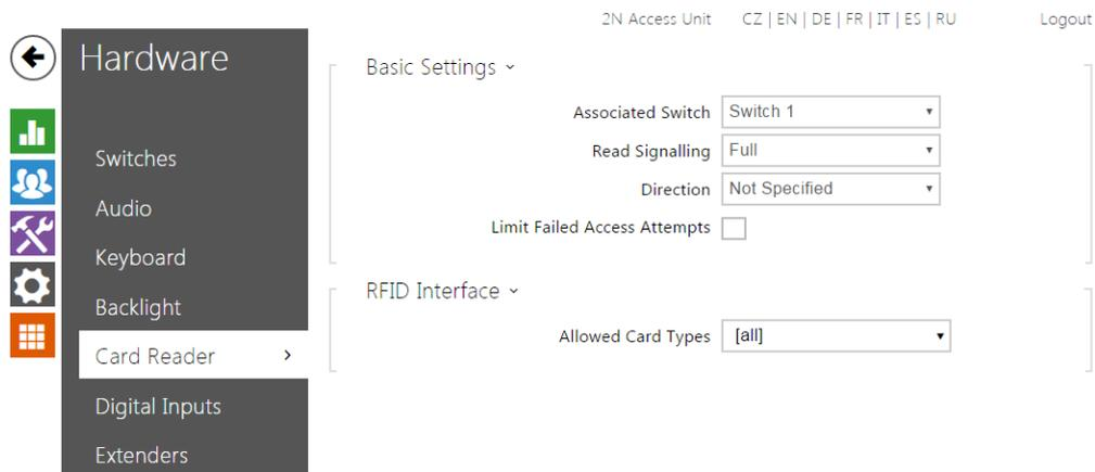
The card reader helps you control access to your building effectively using contactless RFID cards. The supported card types depend on the card reader model used.
