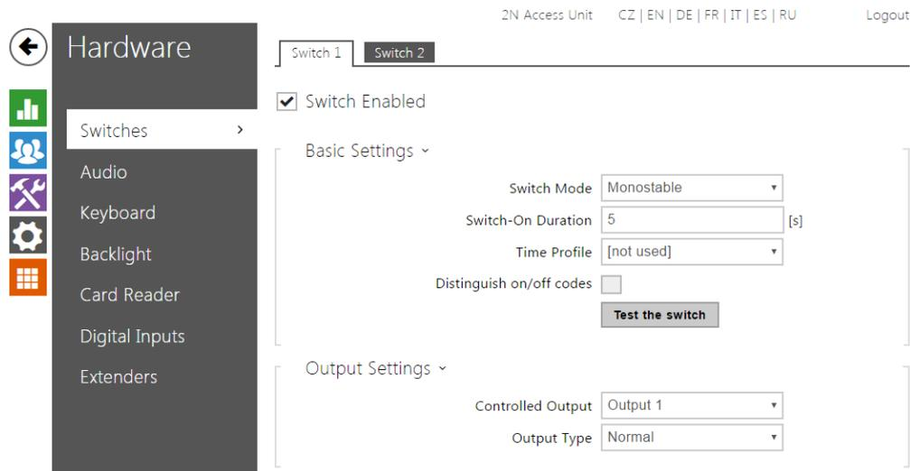
Switches provide a very flexible and efficient control of such peripherals connected to the Access Unit as electric door locks, lighting, additional ringing signalling, and so on.
