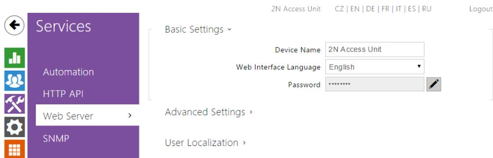
You can configure your **2N<sup>®</sup> Access Unit** using a standard browser with access to the integrated web server. Use the secured HTTPS protocol for communication between the browser and **2N<sup>®</sup> Access Unit**. Having accessed the intercom, enter the login name and password. The default login name and password are **admin** and **2n** respectively. We recommend you to change the default password as soon as possible.
