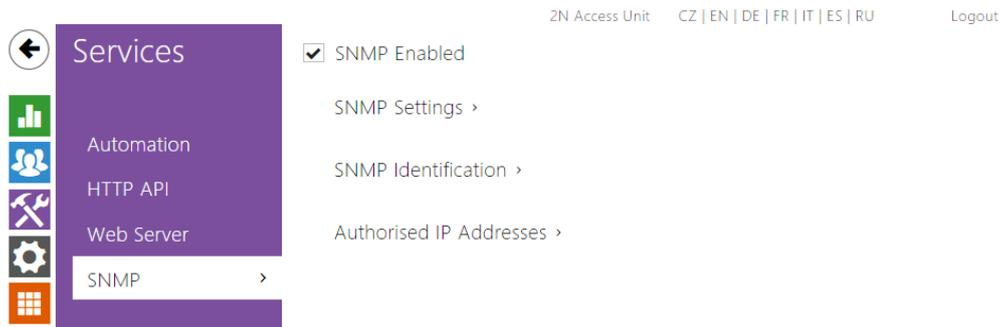
The 2N<sup>®</sup> Access Unit integrate a remote intercom supervision functionality via the SNMP. The 2N<sup>®</sup> Access Unit support the SNMP version 2c.
