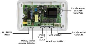
Screw terminal connections for AC Power, AUX Wired Inputs, Loudspeaker Outputs and Line Level outputs are located on the rear PCB of the AVID3ACBT.
