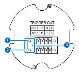
**1** VCC: Connects to the 5v power pin on the connected control system's trigger block.
