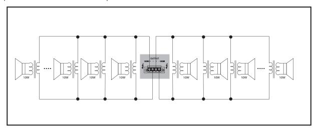
\* Caution: 1. Make sure that the total impedance does not equal or less than the rated impedance.
