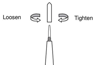
▶ Firmly tighten up the 4mm Tips.
