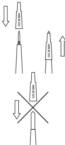
▶ Do not install the CAT.III/IV cap when the 4mm Tips is installed.
