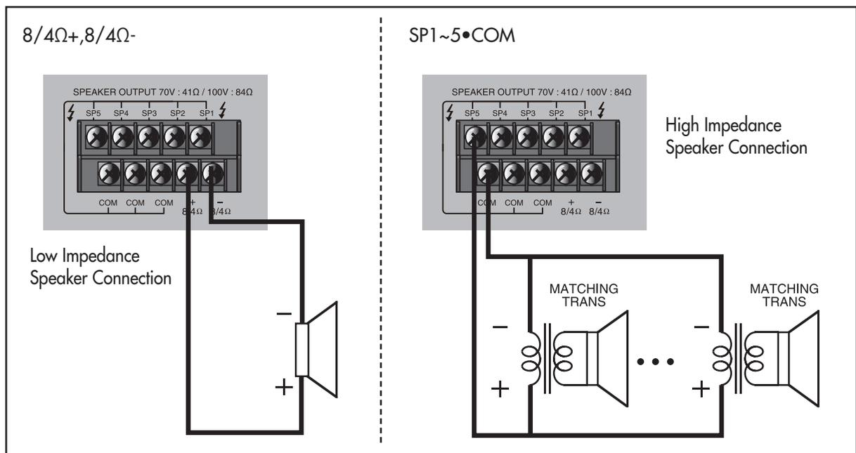
※ Caution: Be careful not to make total impedance of the speaker terminal to be lower than defined impedance in any case. Impedance and output voltage are as the following table:
