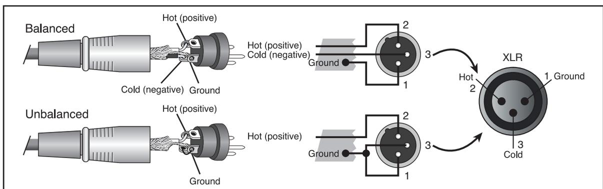
Turn PHANTOM switch OFF if using the unbalanced cable.
