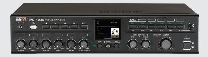
The PMU-120N are 6-Input 120-watt mixer/amplifier with a built in digital portable media player that will playback MP3 / WMA / WAV audio files. The PMU-120N offers input flexibility with its 6 microphone and line level selectable inputs. Direct PC USB connection is possible using the built in USB PC sound card. A network audio connection makes the PMU-120N amplifier great for BGM applications that receive their audio program via network, LAN, WAN and internet TCP/IP or RTSP.
