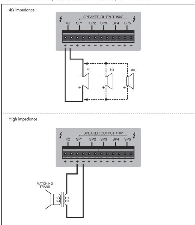
\*Warning: For high impedance systems, connect with matching transformer as the following Figure. Be certain that the total impedance does not equal less than the rated impedance.
