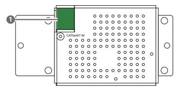
**CAT5e/6/7 IN:** Connect to the Transmitter unit with CAT5e/6/7 cable for transmission of all data signals.
