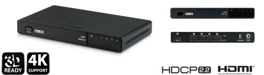
The QU-14S-4K Distribution Amplifier (splitter) accepts one HDMI input and splits this signal to four identical outputs. This device is v1.4 HDMI compliant and supports HDCP 2.2, 3D Video signals and 'Deep Colour', and 4K resolutions, together with High Definition Audio. Each buffered output can run 1080p/8-bit up to 20 metres and can also be cascaded up to 3 layers.
