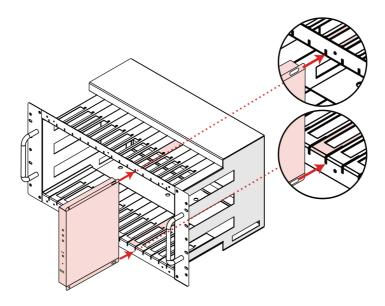
**STEP 3**Reattach the top and bottom locking panels by screwing in the 3 thumbscrews on each until they are tight and secure.
