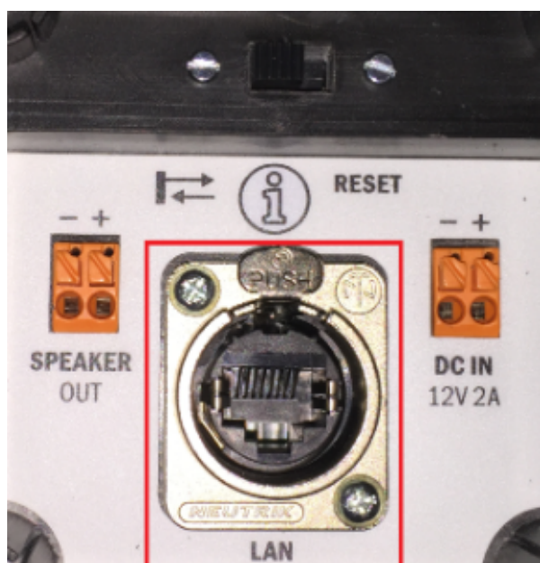
Figure: LAN Connection
